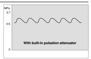
pressure when discharge pressure increases, and compensates the pressure when discharge pressure decreases. By this means pulsation is controlled.
