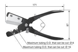
Note) Do not use it to cut the metalic materials such as electric wires.
