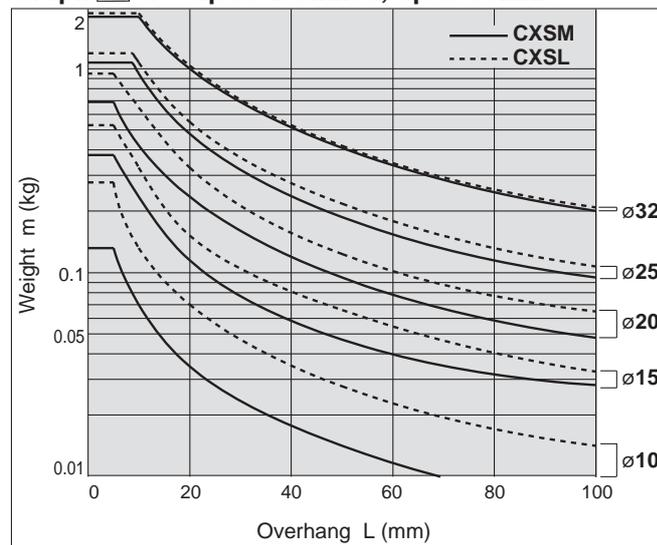
**Horizontal Mounting [based on maximum speed and stroke length]**
