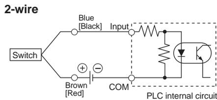
The connection method will vary depending on the applicable PLC input specifications.
