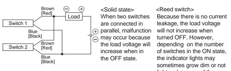
$$\begin{aligned} \text{Load voltage at OFF} &= \text{Leakage current} \times 2 \text{ pcs.} \times \text{Load impedance} \\ &= 1\text{mA} \times 2 \text{ pcs.} \times 3\text{k} \\ &= 6\text{V} \end{aligned}$$
