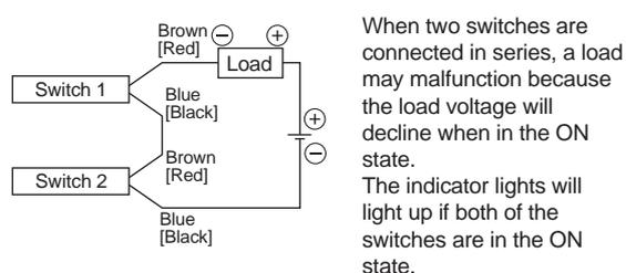
$$\begin{aligned} \text{Load voltage at ON} &= \text{Power supply voltage} - \text{Internal voltage drop} \times 2 \text{ pcs.} \\ &= 24\text{V} - 4\text{V} \times 2 \text{ pcs.} \\ &= 16\text{V} \end{aligned}$$
