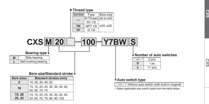
Applicable auto switches: Refer to pages 40 through 48 for detailed auto switch specification
