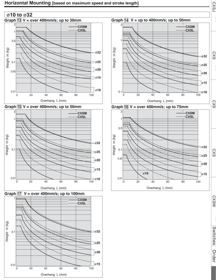
Horizontal Mounting [based on maximum speed and stroke length]
