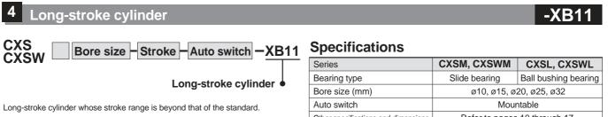
Note) The specification for long-stroke cylinder -XB11 is available within the ranges shown in the table at right. Cylinders with even longer strokes are available as a special order.
