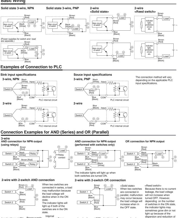
Internal Load voltage at ON = Power supply voltage drop x 2 pcs. voltage = 24V - 4V x 2 pcs. = 16 V
