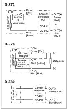
Note) A contact protection box should be used in any of the following conditions to prevent the shortening of the working life of the switch.
