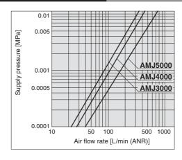
Fluid: Air (pressurised) Measured pressure: Downstream release to atmosphere
