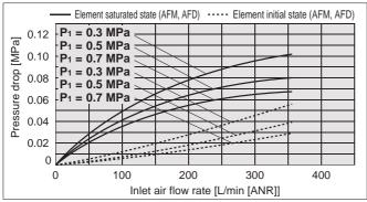
Conditions: Inlet air temperature 25°C, P1: Inlet air pressure
