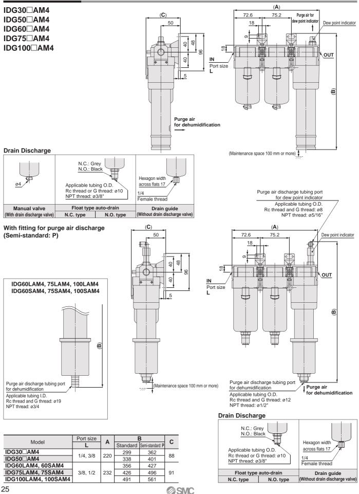
Membrane Air Dryer Unit Type Series IDG A/IDG
