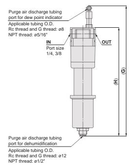
With fitting for purge air discharge (Semi-standard: P)
