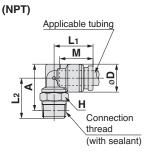
Reference dimensions after installation for NPT thread Note) Value of FEP tubing.
