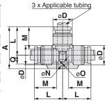
Note 1) For the  $\emptyset$ 16, this dimension refers to the O.D. of the release button. Note 2) Value of FEP tubing.
