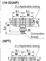
Connection thread (with sealant)
