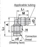
Note 1) For the  $\emptyset$ 16, this dimension refers to the O.D. of the release button. Note 2) Value of FEP tubing.
