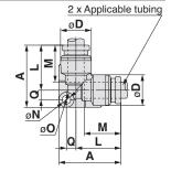
Note 1) For the ø16, this dimension refers to the O.D. of the release button. Note 2) Value of FEP tubing.
