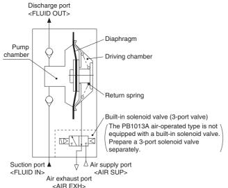
When air is supplied with the built-in solenoid valve turned ON (energized), air enters the driving chamber and the diaphragm moves to the left. Due to this movement, the fluid in the pump chamber passes through the upper check valve and is discharged to the discharge port <FLUID OUT>.
