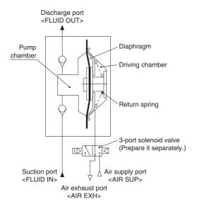
When air is supplied with the external 3-port solenoid valve turned ON (energized), air enters the driving chamber and the diaphragm moves to the left. Due to this movement, the fluid in the pump chamber passes through the upper check valve and is discharged to the discharge port <FLUID OUT>.
