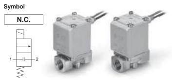
When the valve is closed, flow is blocked from port 1 to port 2. However, if the pressure in port 2 is higher than port 1, the valve will not be able to block the fluid and it will flow from port 2 to port 1.
