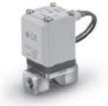
When the valve is closed, flow is blocked from port 1 to port 2. However, if the pressure in port 2 is higher than port 1, the valve will not be able to block the fluid and it will flow from port 2 to port 1.
