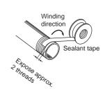
In applications such as vacuum and non-leak specifications, use caution specifically against the contamination of foreign objects or airtightness of the fittings.
