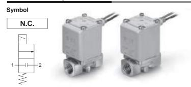
When the valve is closed, flow is blocked from port 1 to port 2. However, if the pressure in port 2 is higher than port 1, the valve will not be able to block the fluid and it will flow from port 2 to port 1.
