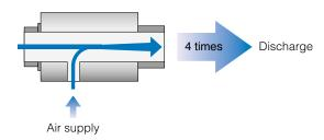
Suctioning is possible at a flow rate triple the supplied air.
