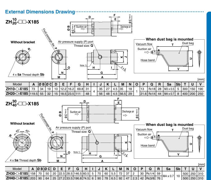
Note 1) This thread portion is intended for use in manufacturing processes. Applying rotational torque to the thread or using it for mounting may result in a change in the characteristics of the product at the time of shipment. Therefore, do not apply rotational torque to the thread or use it for mounting.
