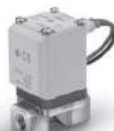
When the valve is closed, flow is blocked from port 1 to port 2. However, if the pressure in port 2 is higher than port 1, the valve will not be able to block the fluid and it will flow from port 2 to port 1.
