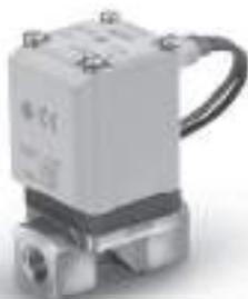
When the valve is closed, flow is blocked from port 1 to port 2. However, if the pressure in port 2 is higher than port 1, the valve will not be able to block the fluid and it will flow from port 2 to port 1.
