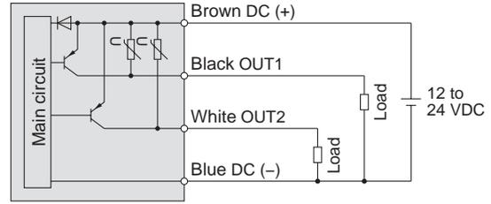
Max. load current: 80 mA, Internal voltage drop: 1.5 V or less
