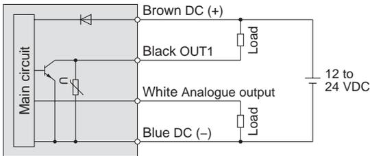
Max. applied voltage: 28 V, Max. load current: 80 mA, Internal voltage drop: 1 V or less
