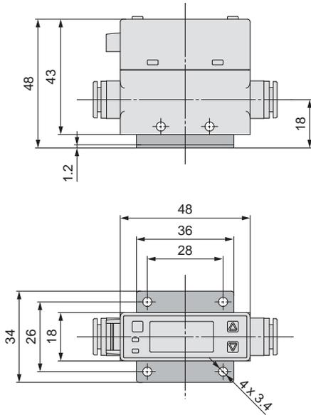
With bracket/With flow adjustment valve
