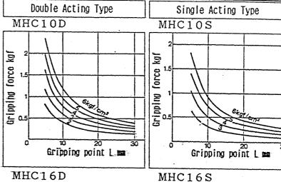
Guidelines for The Selection of Air Chuck Hodel with Respect to Component Weight
