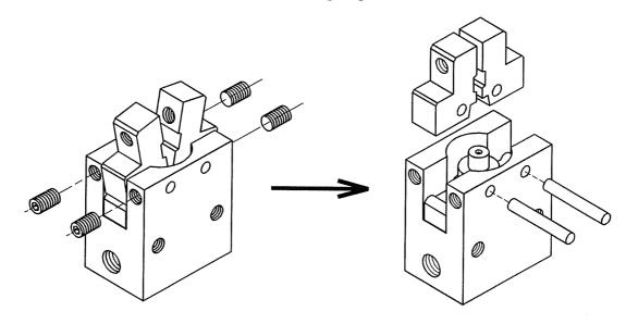
2. Take off pusher, spring and piston and replace packing.
