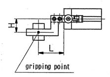
Gripping point; The length of L and length of H should be used within the limits described on P5.
