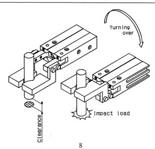
3. Adjust the holding point so that excessive force will not be applied on fingers when inserting the work.
