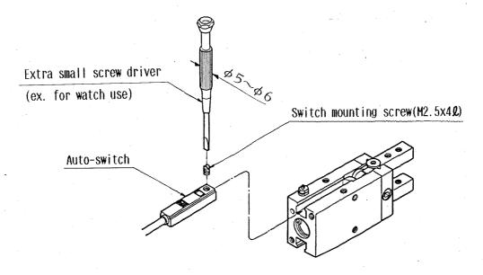
Note) To tighten auto-switch fitting screw, use extra small screw driver of grip dia. approx. 5-6mm. Advised tightening torque is approx.  $0.5-1kgf \cdot cm$ . When touch feeling is obtained, rotate  $90^{\circ}$  to reach the required torque.
