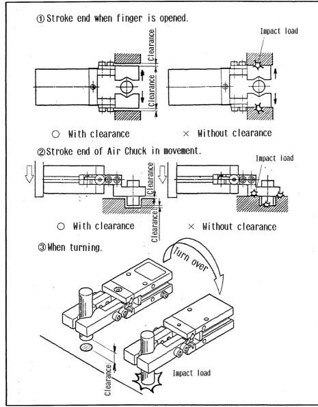
Appropriate clearance should be kept at finger not to receive force except gripping workpiece, particularly when workpiece is gripped, not to crash to other object at stroke end of Air Chuck movement, Lateral load comes on to finger repeatedly or impact load comes on may cause finger to loosening or damage. It is often happens when Air Chuck is turned little variation of length of workpiece may cause to crash at downward stroke end of turning movement. It should be cared.
