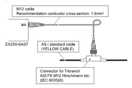
The M12 cable, AS-i standard cable and connector for T-branch are not supplied by SMC. Contact each manufacturer for the catalogue details etc.
