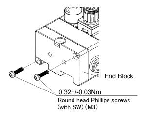
2. Tightening torque of round head combination screw for DIN rail stop ring under regulator manifold specification
