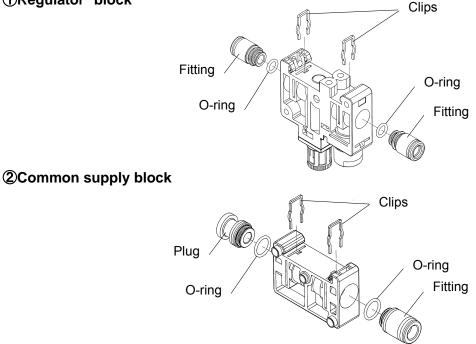
**Exchange of pressure gauge and port plug.** A pressure gange and port plug can also be replaced in accordance with the same replacement procedure of One-touch fittng.
