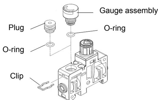
Note 1) Be sure to check that no pressure is supplied from the inlet and outlet ports before replacement, and eliminate the internal pressure completely before starting the operation. It is dangerous if the operation is started with the pressure is sealed inside.
