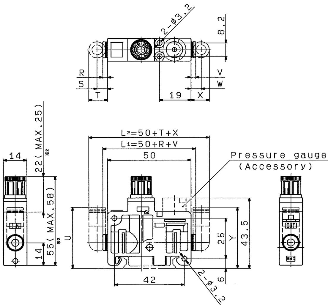
\* 2. MAX dimension indicates the value when handle is unlocked.
