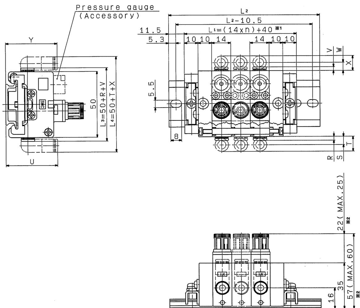
\* 2. MAX dimension indicates the value when handle is unlocked.
