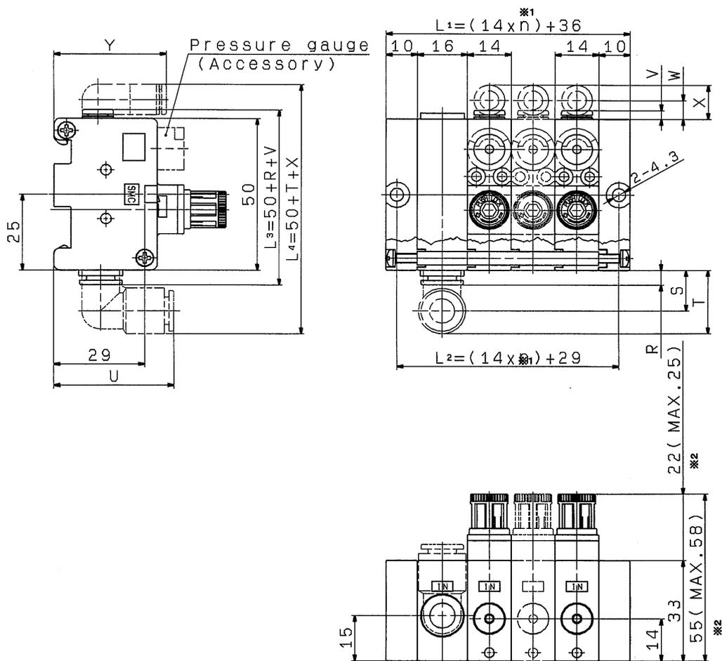
\* 2. MAX dimension indicates the value when handle is unlocked.
