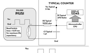
Duty Cycle: THigh / (THigh + TLow) % MODEL FLOW RATE PULSER Fre-/ min. g / min Pulse / liter Pulse / Gal **K24** |5 - 120 | 1,3 - 31,7 379 | 200 Hz | 70 - 90%
