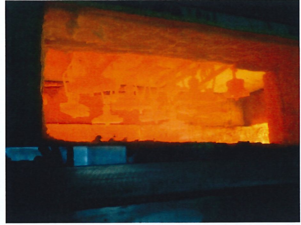
Figure A4.5 View of the clamps in the 75th minute of test.
