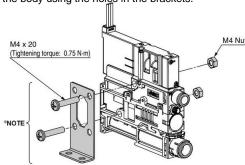
Note) Mounting bracket for single unit (Option) [Nuts and bolts are included.] Part number: ZK2-BK1-A
