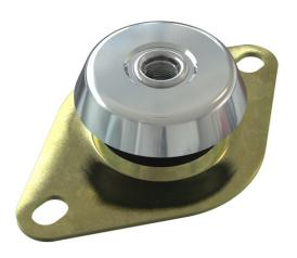
Swerub RAB mountings are used in a wide range of Static and Mobile applications. Characteristics in general similar to SWERUB RA but due to its especially compound the SWERUB RAB is more effective for vibration isolation from 1 - 3 cylinder Diesel Engines and other excessive movements.
