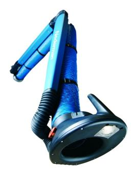
NEX MD welding fume extraction arms are the top of the range arms when it comes to high airflows and extraction of media with higher temperatures than normal. The weld fume extractors are specially designed for working environments with very heavy smoke, vapours or non explosive dust. Typical workplaces are the metal fabrication industry or other type of industries where the need for extraction with large airflows is needed.
