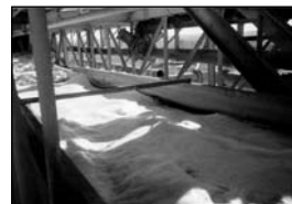
Photo E: TIVAR® 88-2 launderer running full. To date, no signs of wear or corrosion are visible.
