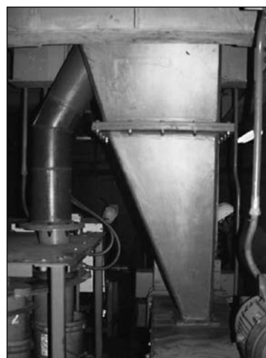
After Sample collector manufactured completely with TIVAR® 88-2 eliminates build-up and quality control problems.
